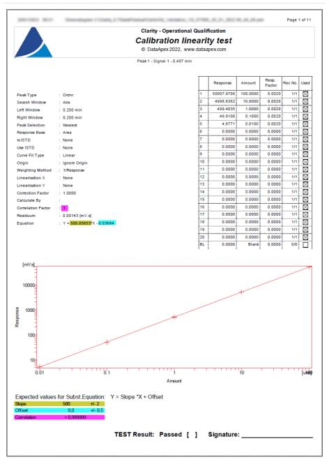
Fig. 2: Calibration linearity test - report
