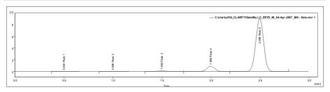
Next six identical chromatograms have **peaks increasing in size by factor of 10**, the last peak has height 9000 mV and area 50000 mV.s. They are used for ESTD calculation and reproducibility tests.
