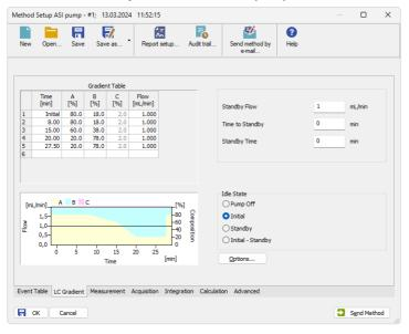
Fig. 6: Method Setup - LC Gradient
