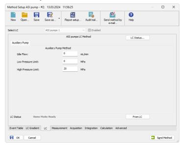
Fig. 8: Method Setup - LC - Auxiliary Pump
