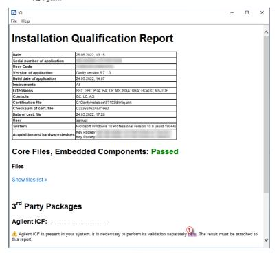
Click the link "here" ①, after that it is necessary to click Run in two pop-up windows. Agilent Software Verification Tool window will open. Select what report file type should be generated and define post-qualification actions. Click Qualify ② to run the IQ. The HTML reports are opened in the default browser if the Open reports option was enabled. Installed drivers and their versions are listed at the end of the report.
