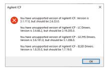
Fig. 29: An Agilent ICF error during Clarity start
