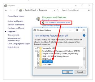
Fig. 6: Windows 10 - Telnet client
