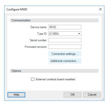
Fig. 15: Example of configuring the MWD
