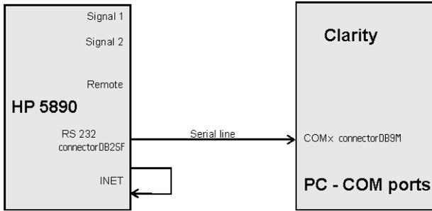
When the **HP5890** is controlled by the serial line (**RS232**), both **INET** connectors must be connected, which can be done by wiring on the back side of the card or INET loop cable.
