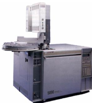
Fig 1: Agilent (HP) 5890 with an autosampler
