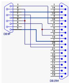
*Fig 3: Serial cross cable DB9F - DB25M*
