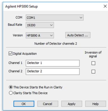
Fig 5: Agilent HP5890 Setup
