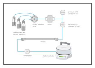
Fig. 4 - Diagram of the Stacked Injection SEC system
