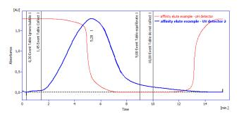
*Fig. 2 - Example of the elution cycle in immunoaffinity separation*
