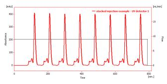
Fig. 6 - Example of stacked injection SEC separation
