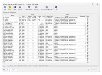
Fig. 5 - Example of Stacked Injection Method Event Table
