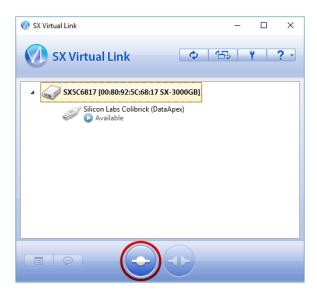
4. If the connection is successful, you will see the USB device in the Windows Device Manager, and you can then configure it in Clarity in the same manner as if it was connected directly to the local computer.
