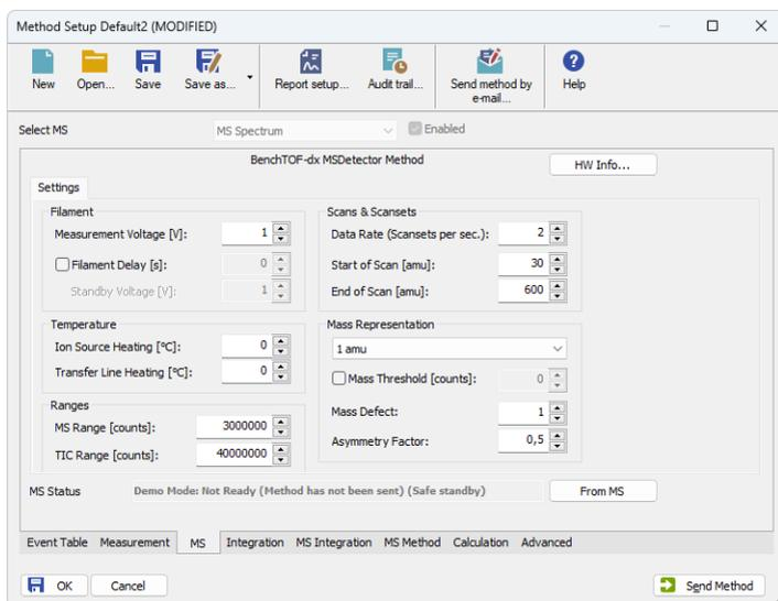
Fig. 4: Method Setup - MS
