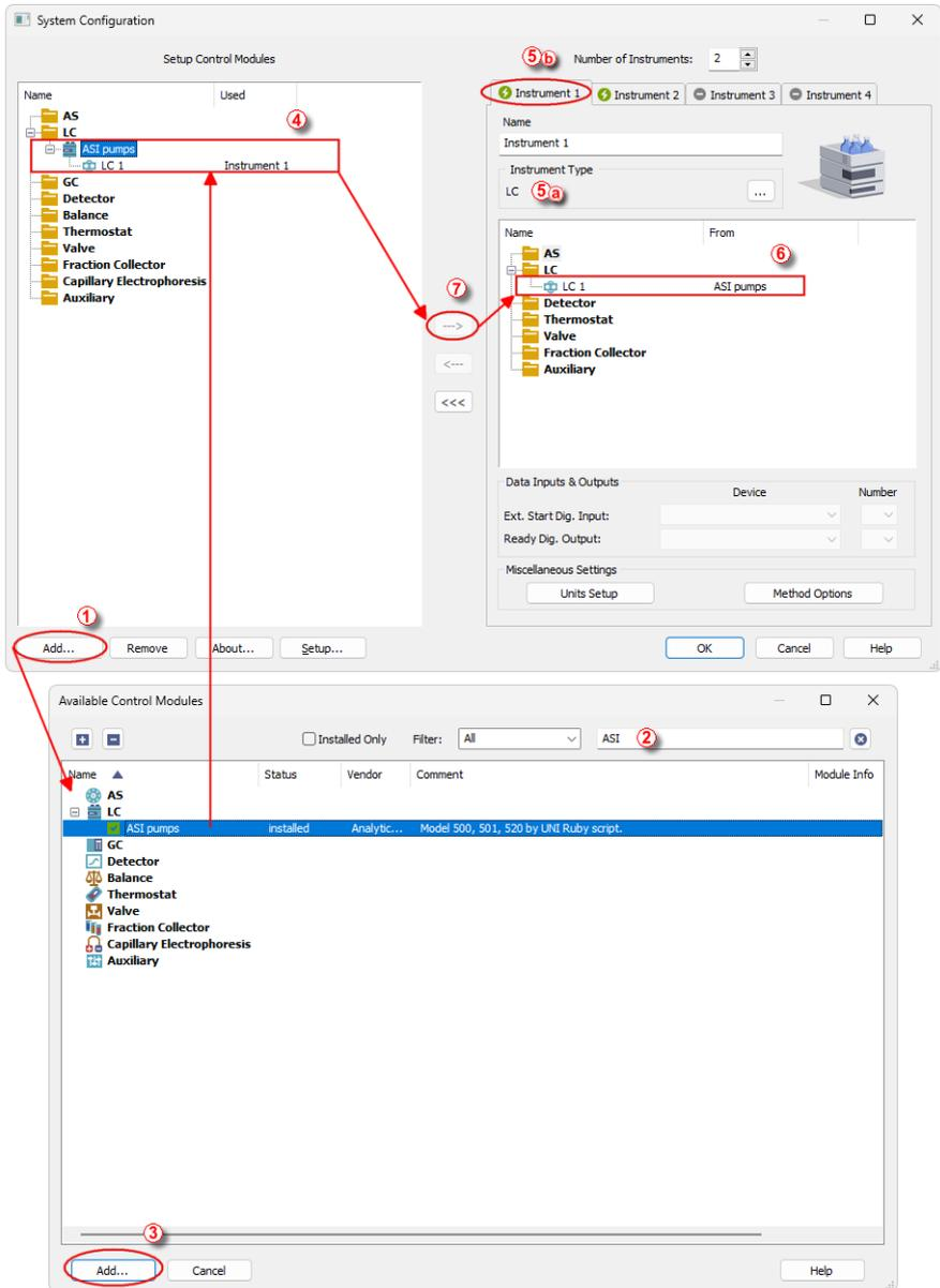
Fig. 4: How to Add ASI Series 500 pumps module
