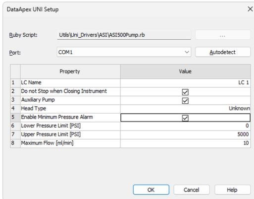
Fig. 11: Hardware Configuration
