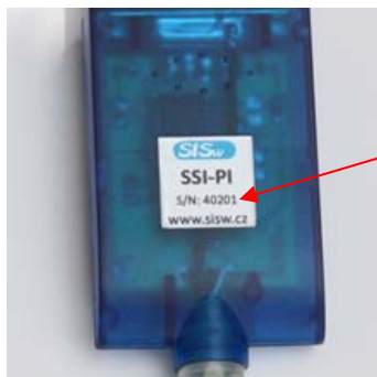
Serial numbers on the interface label and in the port list are identical
