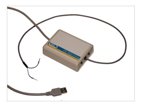
Direct control means that the vacuum measuring activity is fully controlled from Clarity environment. Measured vacuum data may be permanently stored in the measured chromatograms.
