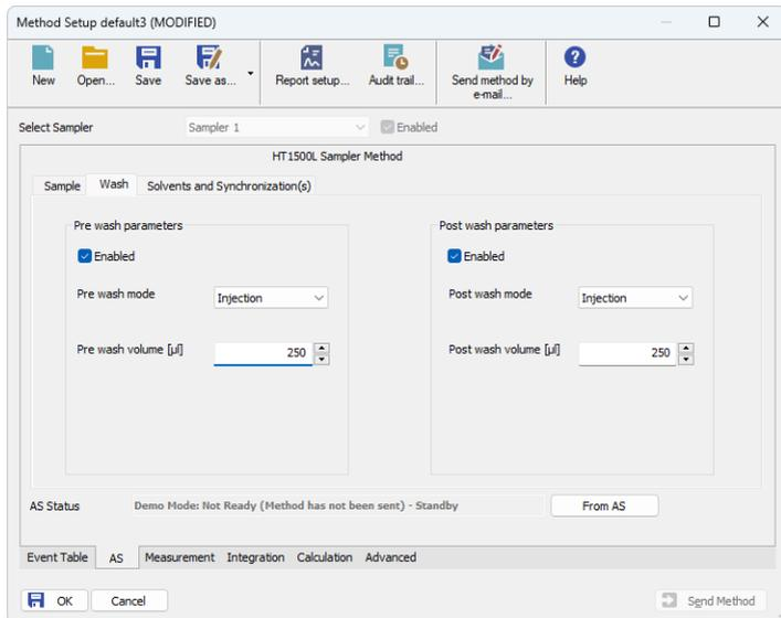
Fig. 5: Method Setup - AS - Solvent Wash
