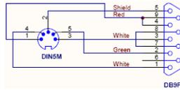
Fig. 2: DB9F-DIN5M cable
