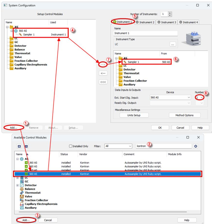
Fig. 3: How to Add Kontron 360/560 module
