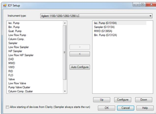
Fig 18: Setup dialog of the Agilent ICF
