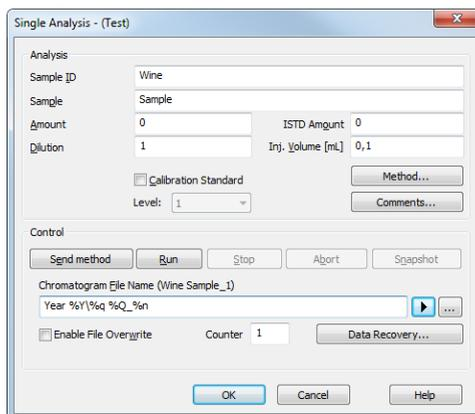
Fig 3: Single Analysis dialog and an example of subdirectory in the chromatogram file name
