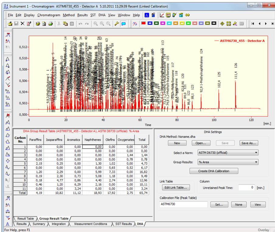
Fig 16: DHA Extension in the Chromatogram window
