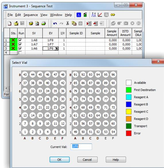
Fig 12: Selecting a vial interactively in the Sequence window
