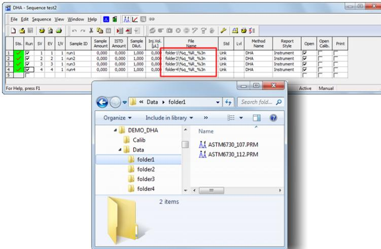
Fig 13: Example of creating subfolders in the Sequence
