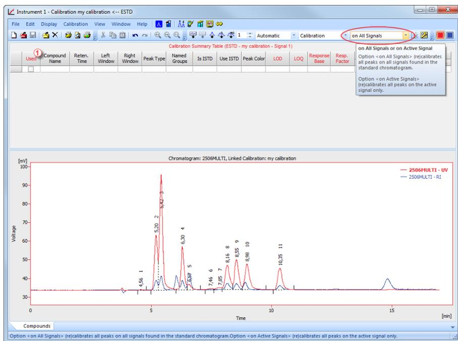
Fig 1: Calibration - on All Signals
