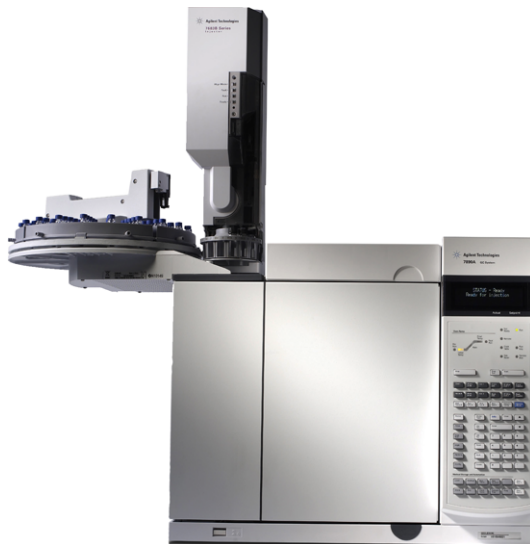
Fig. 1: Agilent 7890A Gas Chromatograph (with 7683 autosampler)
