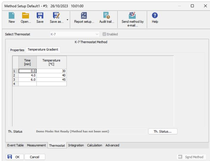
Fig. 6: Method Setup - Thermostat - Temperature Gradient
