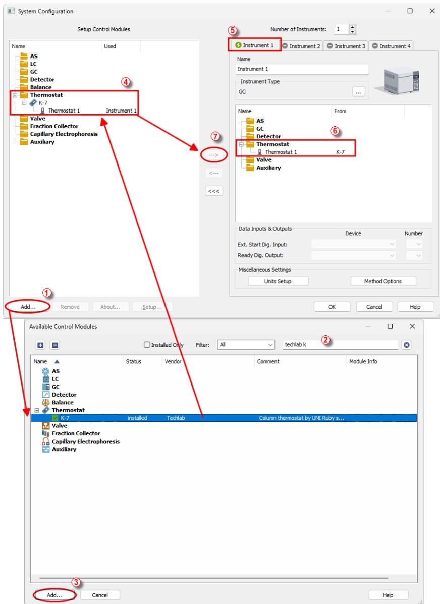
Fig. 3: How to Add Techlab K-7
