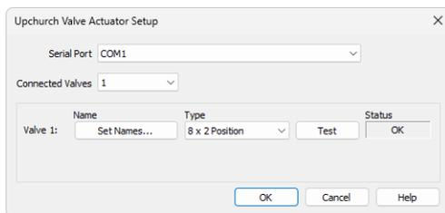
Fig. 8: Upchurch Valve Actuator Setup - 1 connected valve
