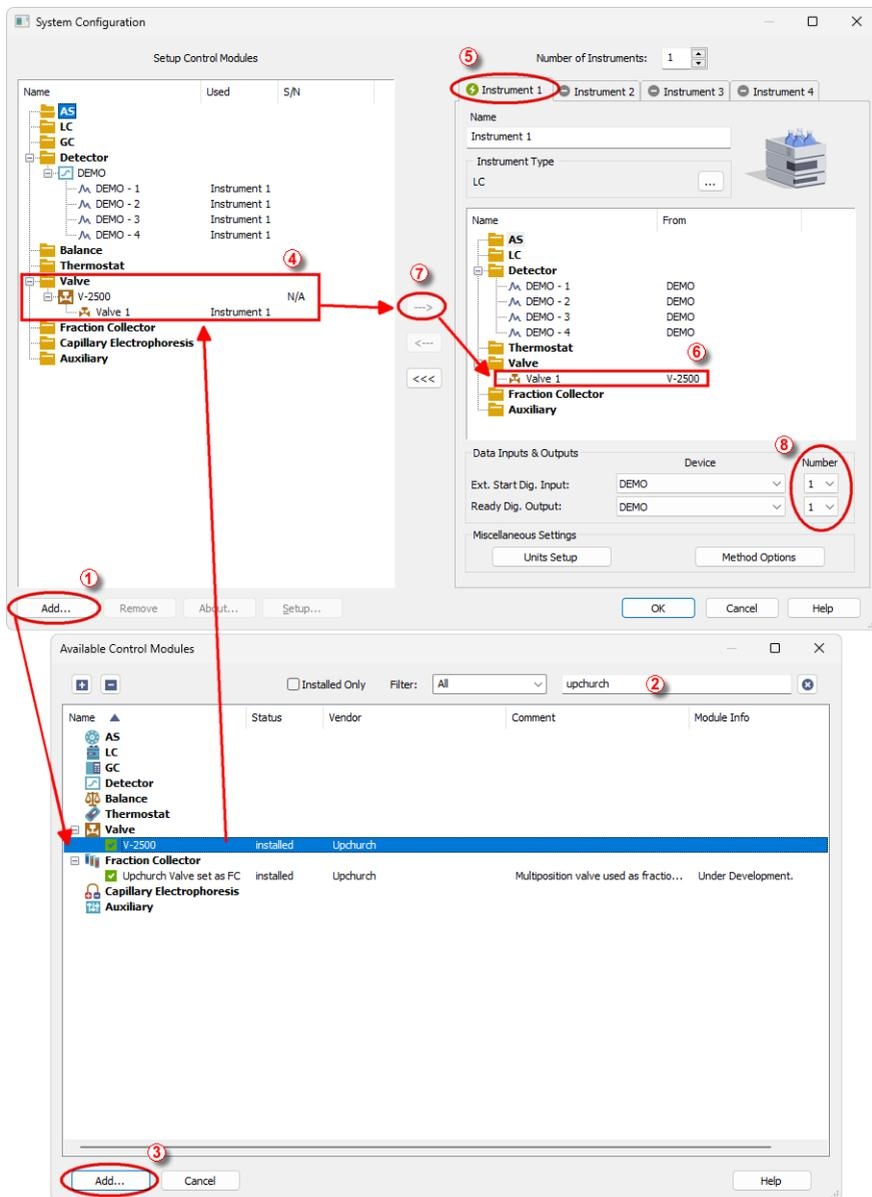
Fig. 2: System Configuration
