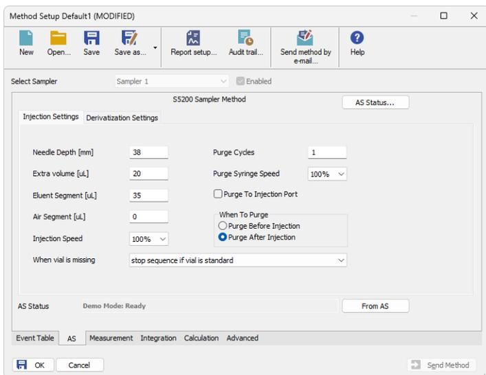
Fig. 6: Method Setup - AS - Injection Settings
