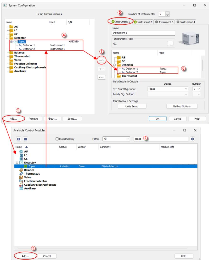
Fig. 4: System Configuration
