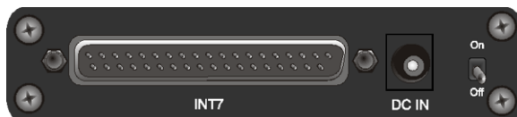
Fig. 4: The right side of the Net-PAD
