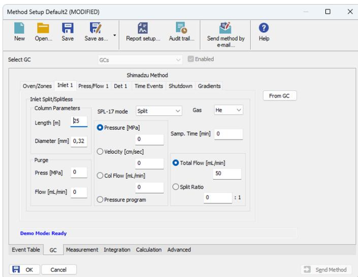
Fig. 7: Method Setup - GC Control - Inlet
