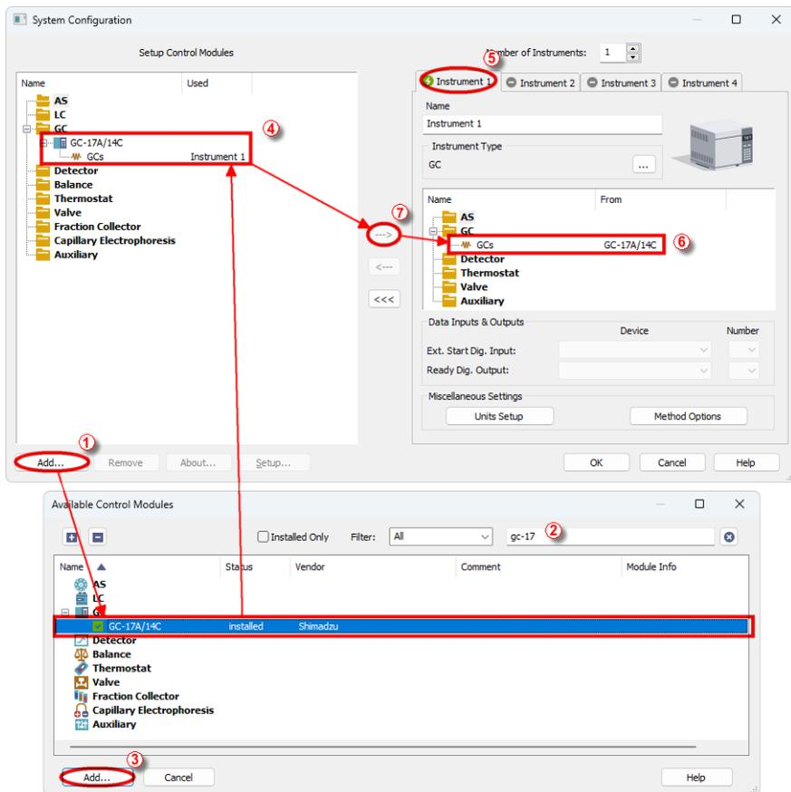
Fig. 4: System Configuration
