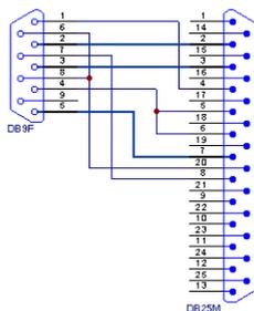
Fig. 3: Serial cross cable DB9F - DB25M
