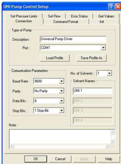
Fig 9: UNI Pump Control Setup - Connection tab
