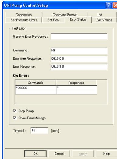
Fig 15: UNI Pump Control Setup - Error Status
