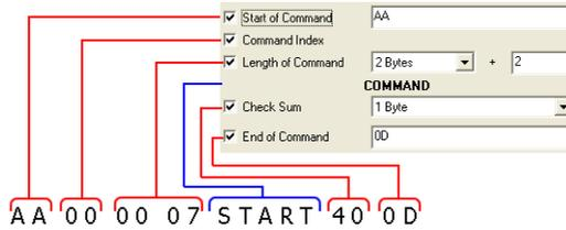
The shell of the command (red) is entered in hexmode and its format will be common to all commands.
