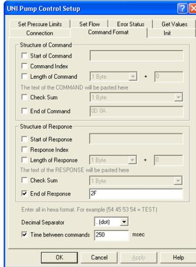
Fig 10: UNI Pump Control Setup - Command Format
