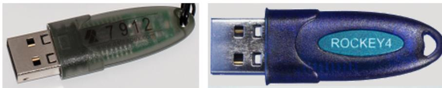
Fig. 21: Current (left) and older (right) hardware key
