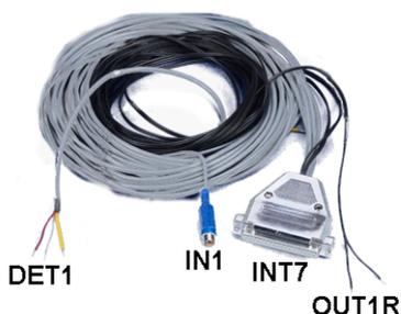
4. Connect the cables (Starting, Digital output and Analog Signal) to the chromatograph as explained in *Connecting a chromatograph analogue output to Clarity*.
