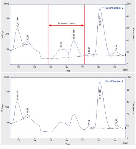
Fig. 135: Peak deletion using Lock
