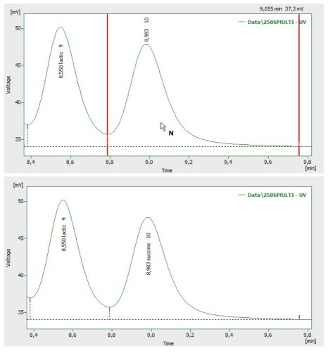
Fig. 156: Override peak name from calibration
