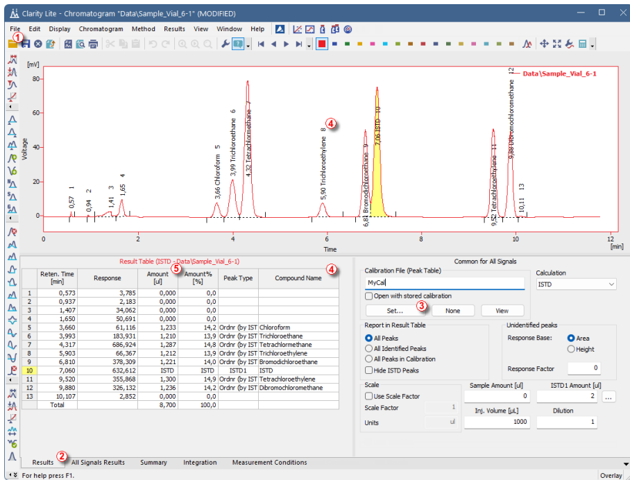
Fig. 14: Calibration linked to chromatogram in the Chromatogram window
