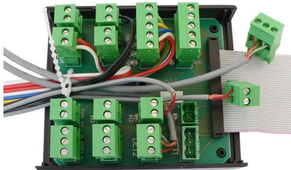
*The individual connectors can be taken out, and LEDs indicate the state of the inputs/outputs*
