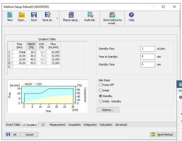
The user can easily create a gradient method from the LC control window and set up a percentage of each gradient component including an overall flow rate in the gradient table. All parameters including parameters controlling pump behavior in the Idle state are a part of the method. Therefore it is possible to create various gradient profiles and choose - only by loading - the corresponding method.
