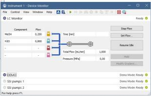
Actual flow rates of each gradient component, their overall sum and pressure can be monitored in the independent LC Monitor. The control is realized via a standard RS232 serial port (one per each pump, Q-Grad requires 4 com ports) using a serial DB9F-RJ11 cable to be ordered with the Clarity Chromatography Station.
