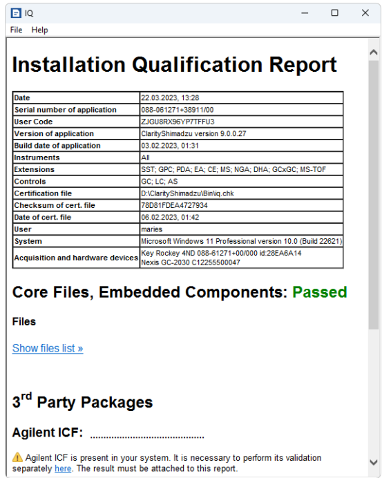
Fig. 8: IQ Report with ICF installation present
