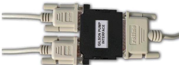
IGLN1 – RS232/GSIOC converter for Gilson
