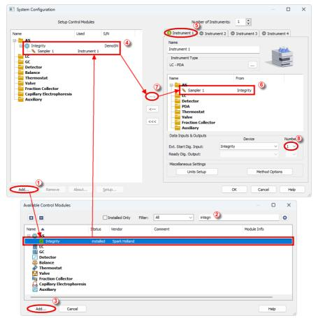
Fig. 5: System Configuration
