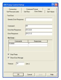
Fig 15: UNI Pump Control Setup - Error Status
