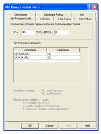
Fig 13: UNI Pump Control Setup - Set Pressure Limits
