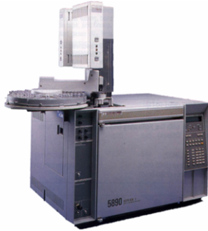
Fig. 1: Agilent (HP) 7673 with a 5890GC
