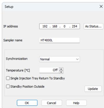
Fig. 12: HTA HT4000L Setup
